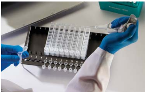
Figure 1. Setup and configuration of the deck tray. Elution Buffer is added to the elution tubes. Plungers are in well #8 of the cartridge. Plasma sample is added to well #1 of the cartridge.
